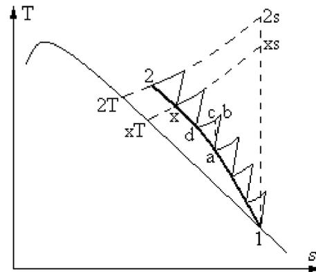
Figure 2 T-s diagram of the simulated compression process
