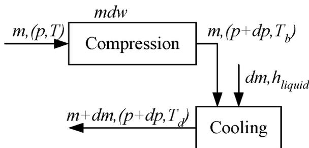
Figure 3 Flow diagram of the infinitesimal process
